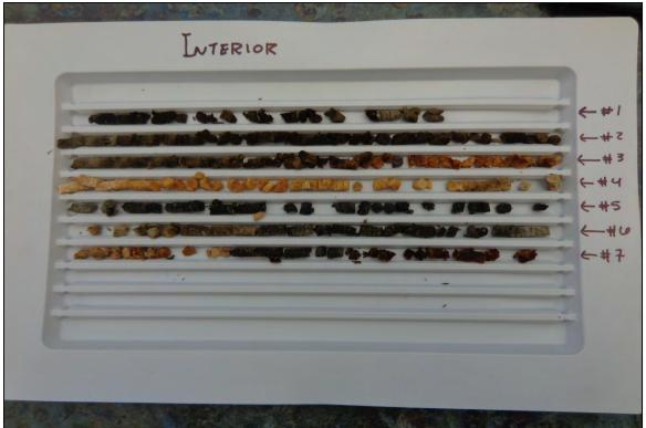
Photograph 29: View of increment core numbers 1 through 7 from the dock interior. Note that these cores fell apart upon removal from coring tool. These do not represent loss of section in the piles.
