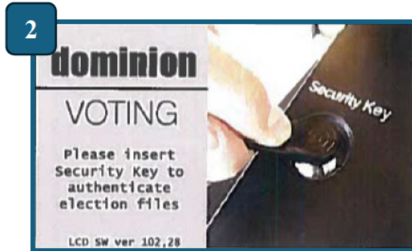
2 – Insert the security key into the security keypad and hold it there firmly until it is accepted
